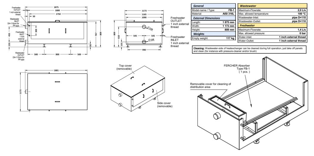
(250403) Datasheet - FERCHER Wastewater-Heatexchanger Type FB-1 - Dimensions and data, all measures in millimeters
