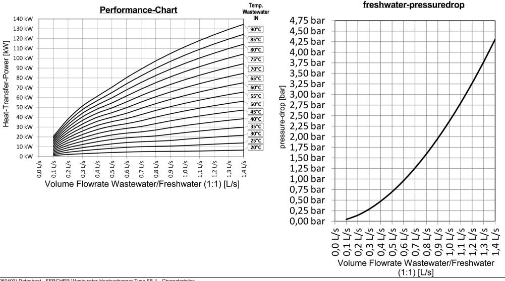
(250403) Datasheet - FERCHER Wastewater-Heatexchanger Type FB-1 - Characteristics
