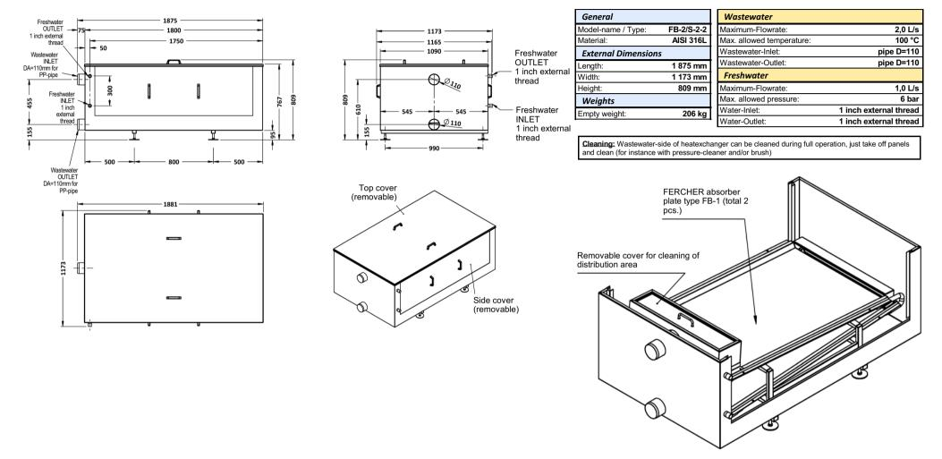
(250403) Datasheet - FERCHER Wastewater-Heatexchanger Type FB-2/S-2-2 - Dimensions and data, all measures in millimeters
