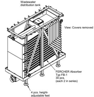
(250403) Datasheet - FERCHER Wastewater-Heatexchanger Type FB-30/W-2-2 - Dimensions and data, all measures in millimeters
