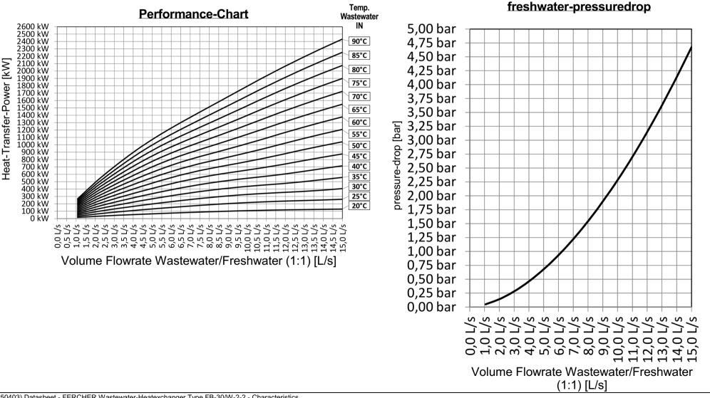
(250403) Datasheet - FERCHER Wastewater-Heatexchanger Type FB-30/W-2-2 - Characteristics
