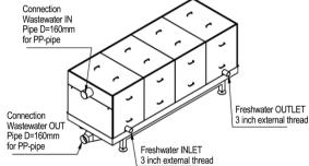
Cleaning: Wastewater-side of heatexchanger can be cleaned during full operation, just take off panels and clean (for instance with pressure-cleaner and/or brush)
